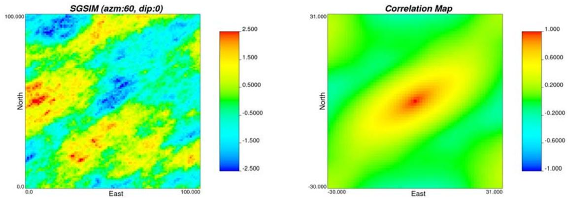
**Figure 2:** A synthetic continues model generated with azimuth of 60 (left) and the calculated correlation map (right).
